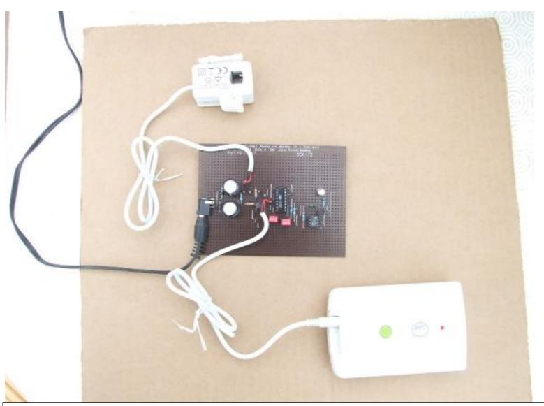
View showing the circuit board connected to the power supply (left) Owl current sensor (top) and transmitter (bottom).
